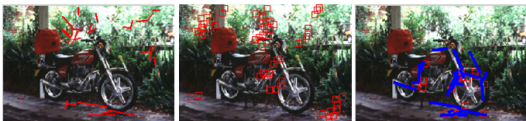
Figure 2. Detections using boundary segments (left), keypoints (center) and combining boundary segments and keypoints (right).
