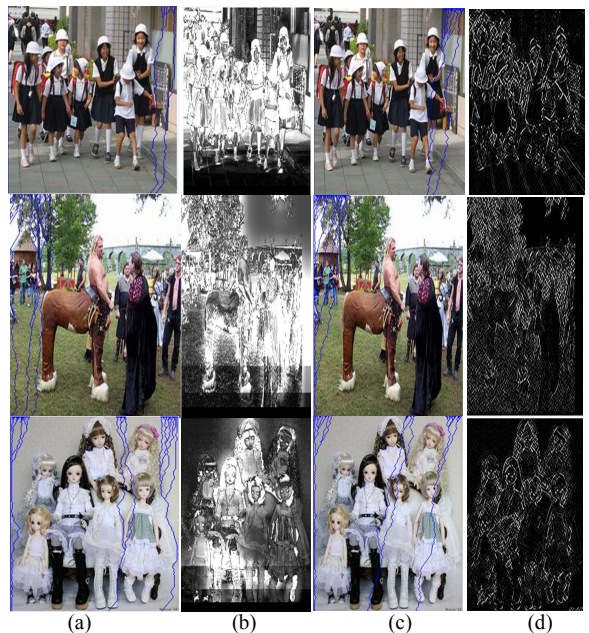
Figure 5. Column (a) and (c) shows original images with less energy stitching lines calculated by corresponding improved energy maps and gradient maps in Column (b) and (d), respectively.
