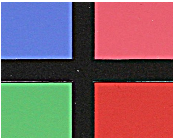
Figure 2. A 1:1 crop of the Macbeth color checker sharpened using unsharp masking with the same settings as those used in the results of figure 1. As seen, the results exhibit edge artifacts and color changes near the borders. The sharpening kernel is 5 \times 5 .
