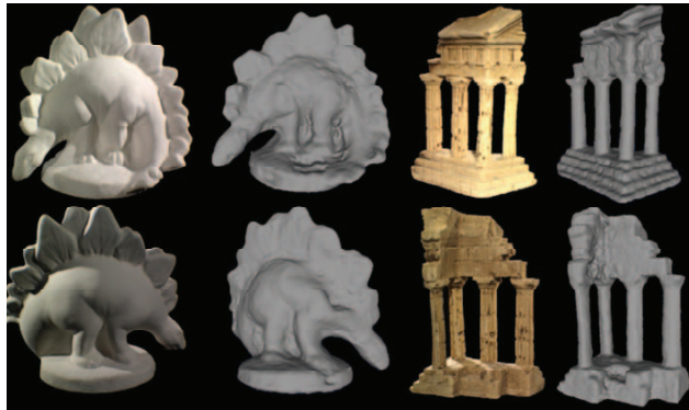
Figure 2. Reconstruction results. First column: 2 of the 16 images in dinoSparseRing. Second column: Reconstruction results of dinosaur in front and back view. Third column: 2 of the 16 images in templeSparseRing. Fourth column: Reconstruction results of temple in front and back view.
