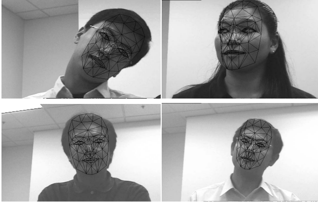
Figure 4. 3D face pose and person-specific shape estimation associated with four unseen persons.
