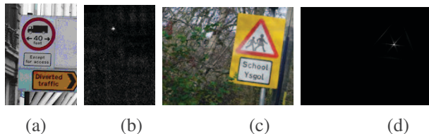
Fig. 2. (a) An input image, (b) its voting image when r = 11 for circular sign detection; (c) an input image, and (d) its shape response image when r = 15 for triangular sign detection.
