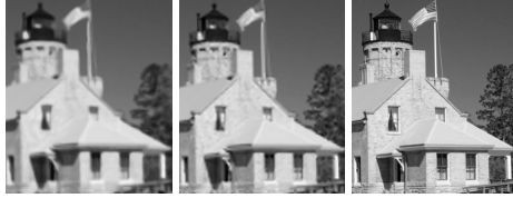
Figure 2. Detail of an image of the test dataset enlarged by a factor 4. IPI (center) provides estimated high frequency details clearly closer to the real ones (right) than those provided by other edge-based method such as improved NEDI (left).
