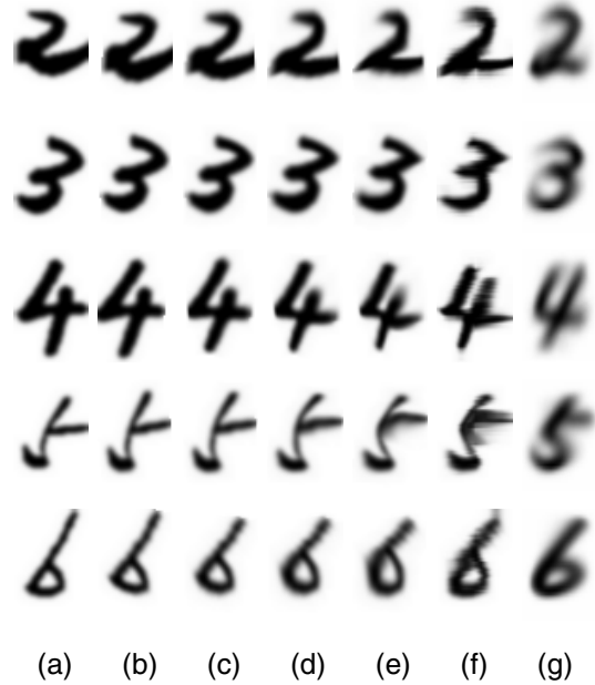
Figure 3. Examples of hierarchical decomposition of DVF. (a) Input images. (b) Global affine transformation. (c) - (e) Successive local affine transformations with \theta = 16, 8, and 4 . (f) PL2DW. (g) Target images.
